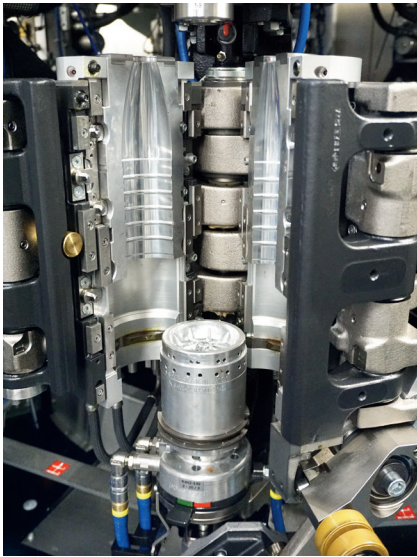
The thumb-sized preforms are "blown up" with a pressure of up to 40 bar.
