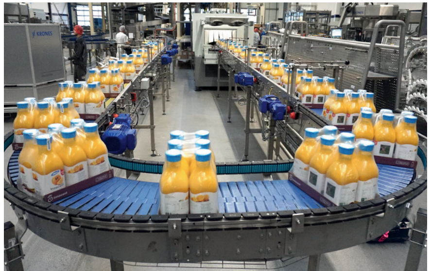
Bottling plant for not-from-concentrate juices at the new plant of the Gropper group of companies in Stockach
