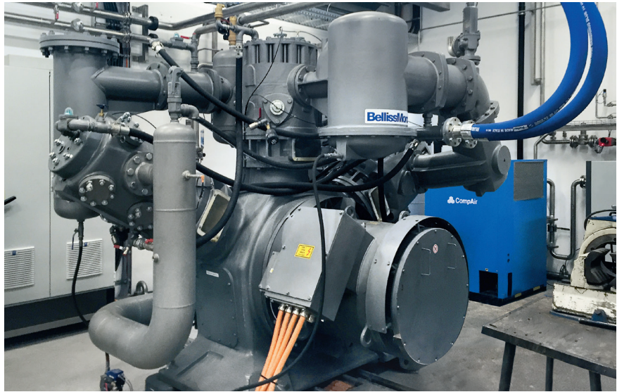
Type WH 29 3N oil-free piston compressor, directly driven with shaftless 325 kW motor, and maximum volume flow of 1,800 m 3 /h (at 40 bar)
